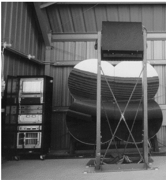
Fig. 6. A prototype mirror unit at HiRes 2. The 2 m diameter mirror is viewed by a cluster of 256 photomultiplier tubes. The rack shown contains the mirror data acquisition crate, power supplies and high-voltage distribution.
