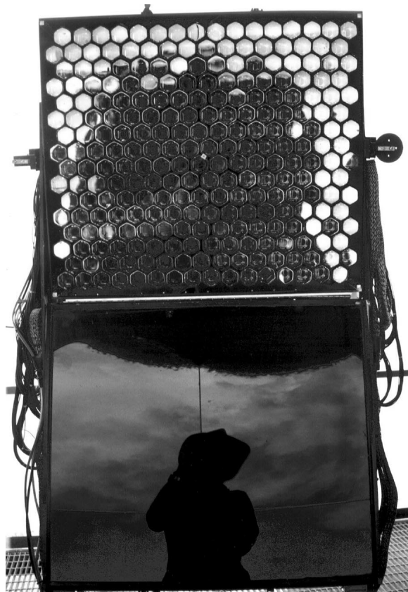
Fig. 7. One of the photomultiplier clusters used to image the night sky. Each cluster consists of 256 40 mm diameter hexagonal photomultiplier tubes each having a 1° field of view. The UV bandpass filter (bottom of picture) has been swung down to reveal the photomultipliers.
