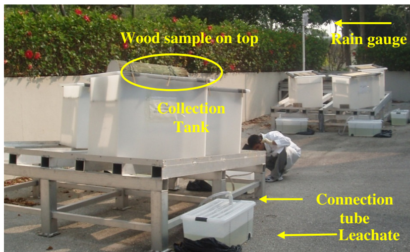
Figure A.1 The experimental leachate-collection systems.
