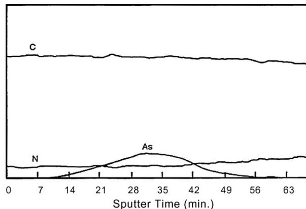
Fig. 1. Auger depth profile of arsenic implanted PAN435. Sputtering rate is 65 Å/min.
