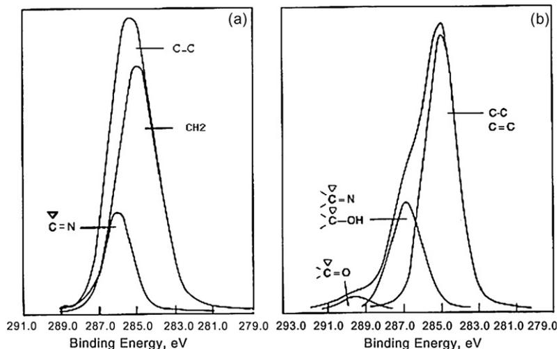
Fig. 3. Curve-resolved XPS C 1s of (a) PAN and (b) PAN435.
