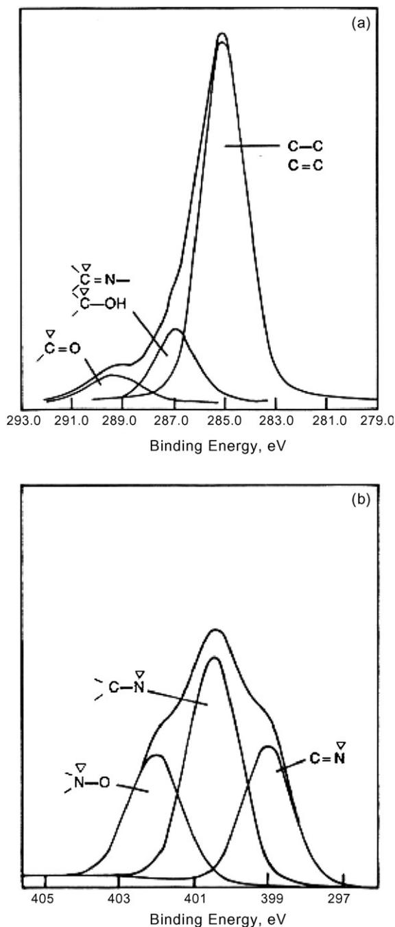
Fig. 5. Curve-resolved XPS (a) C 1s and (b) N 1s spectra of PAN750I.
