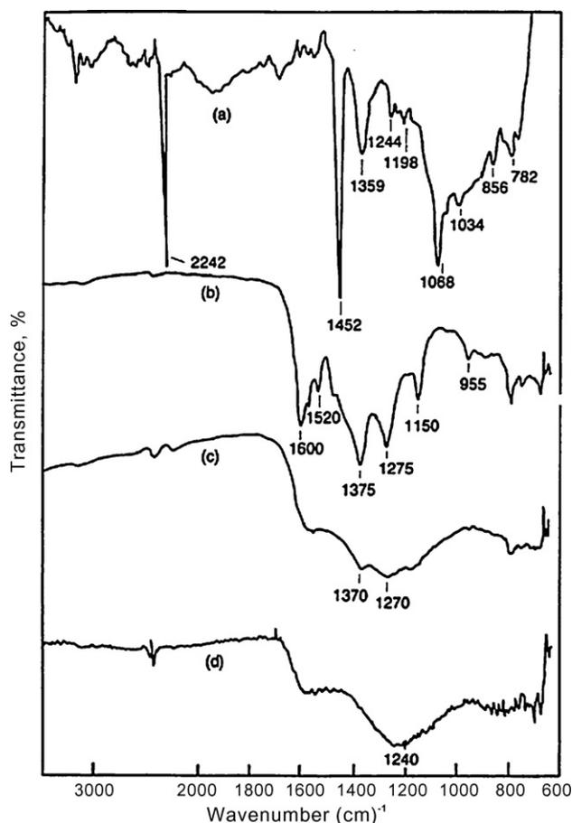
Fig. 2. ATR-FTIR spectra of (a) PAN, (b) PAN435, (c) PAN435I, and (d) PAN750.
