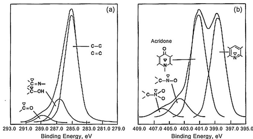
**Fig. 4.** Curve-resolved XPS (a) C 1s and (b) N 1s spectra of PAN750.
