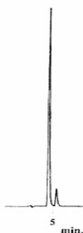
Figure 3. A Chromatogram of Cefotetan disodium solution that was decomposed by use of heat and 0.01M NaOH.
