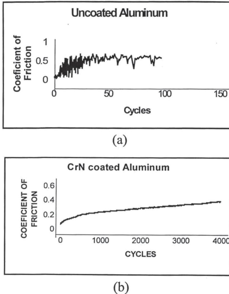
FIGURE 6 Friction traces for coated (a) and uncoated (b) aluminum 6061 disks.
