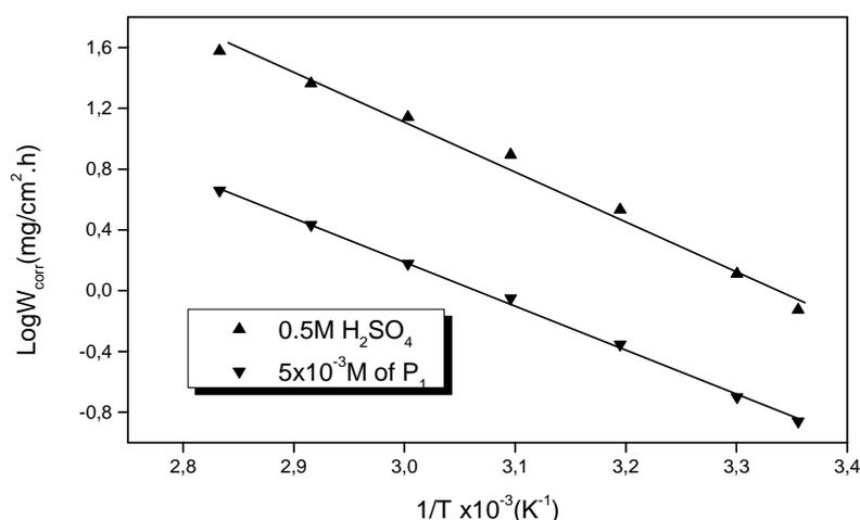
The logarithm of the corrosion rate of steel  $W_{\text{corr}}$  can be represented as a straight-line function of  $1000/T$  (Arrhenius equation, Fig.7), where  $T$  is the temperature in Kelvin:
