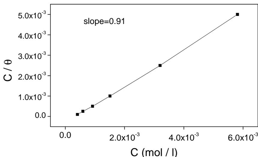
Fig. 8. Langmuir isotherm adsorption of pyrrolidone on steel in 0.5 M  $H_2SO_4$ .
