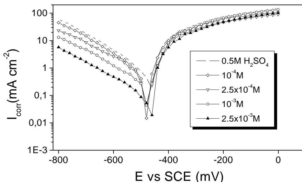
Fig. 3. Polarisation curves of steel in 0.5 M H<sub>2</sub>SO<sub>4</sub> for various concentrations of P1
