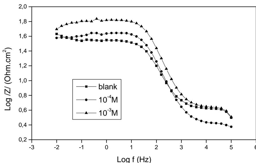
**Fig. 5.** Bode plots of steel in 0.5 M H<sub>2</sub>SO<sub>4</sub> containing various concentrations of P1.
