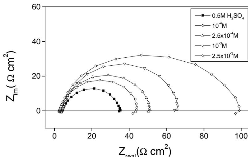
**Fig. 4.** Nyquist plots of steel in 0.5 M H<sub>2</sub>SO<sub>4</sub> containing various concentrations of P1
