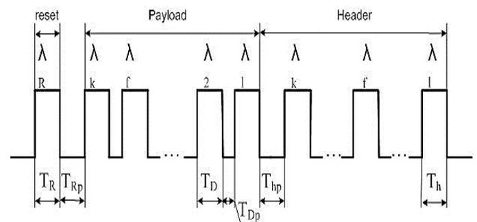
**Figure 7:** Format of the packet.
