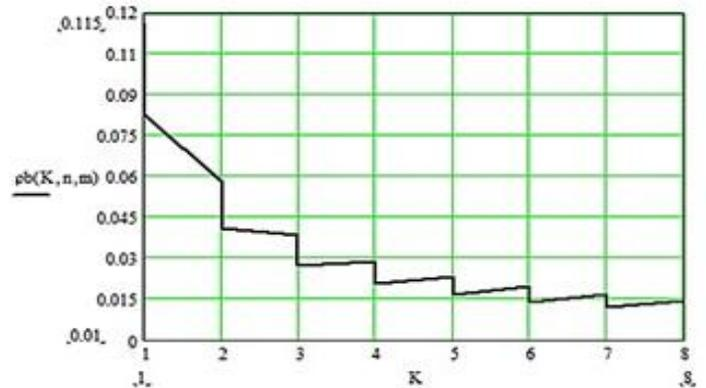
**Figure 10:** Dependence of switchboard load on quantity of auxiliary layers ( $K=8$ ).
