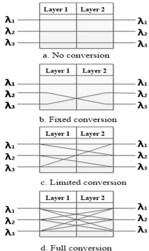
**Figure 3:** Wavelength conversion types.
