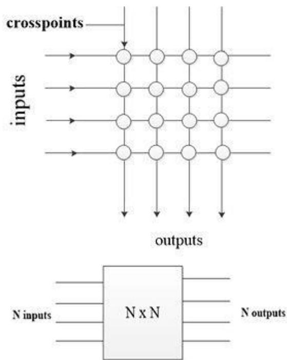
Figure 1:  $N \times N$  Crossbar switch concept.
