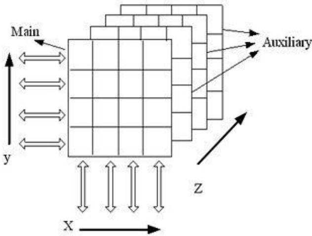
**Figure 5:** Multi-layered architecture of switching matrix.
