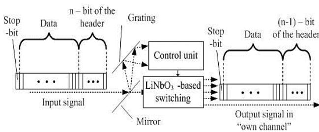
**Figure 9:** Switching of the packets in switchboard.
