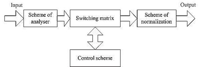
Figure 4: Structural scheme of switch.
