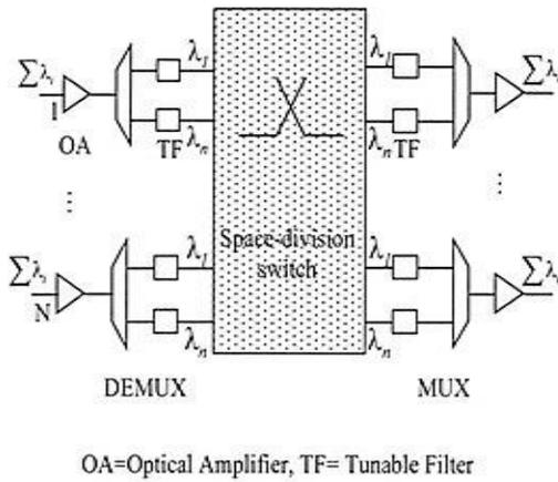
**Figure 2:** Architecture of an optical cross connect.
