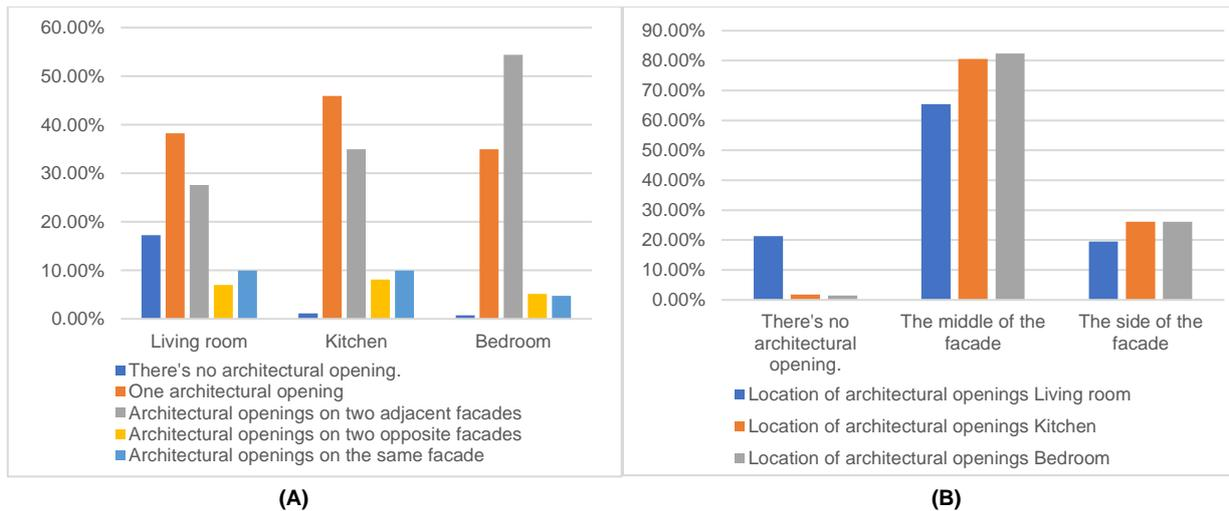
Figure (3): Window's position: (A) windows distribution in the space and (B) windows location in the facade according to the space.
