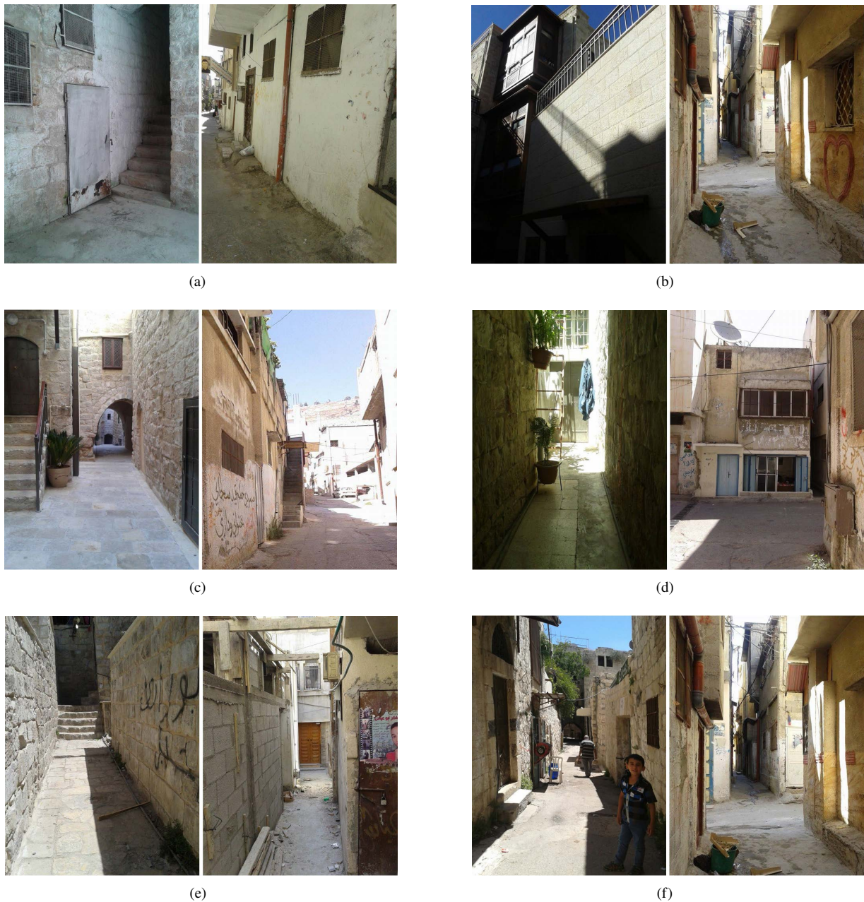
Figure 6. Impact of socio-cultural values on streets design in both old city and refugee camp: (a) Elevated windows from the street level; (b) Using traditional balconies (Meshrabiya); (c) Rising the entrance of the house using stairs;(d) Narrow dead-end streets for house entrances; (e) Minimum opening to narrow pathways; (f) Avoiding in-front entrances
