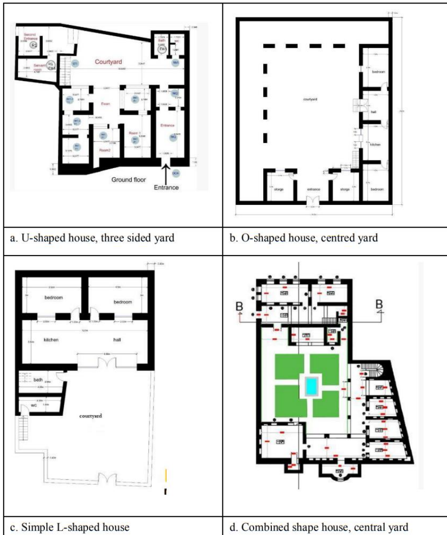
Figure 5. Forms of traditional courtyard housing in Koya City in terms of their relation to the outdoors
