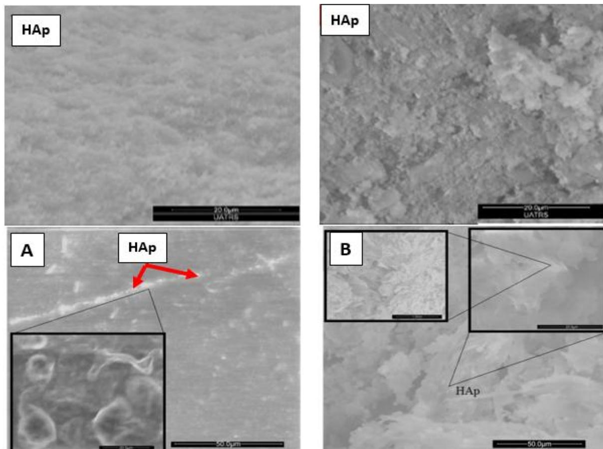
**Figure 4:** SEM micrographs of two membranes surfaces of HAp<sub>t</sub>/PLA/PCL with a molar ratio of a = 50/50/00 and b =50/20/30.
