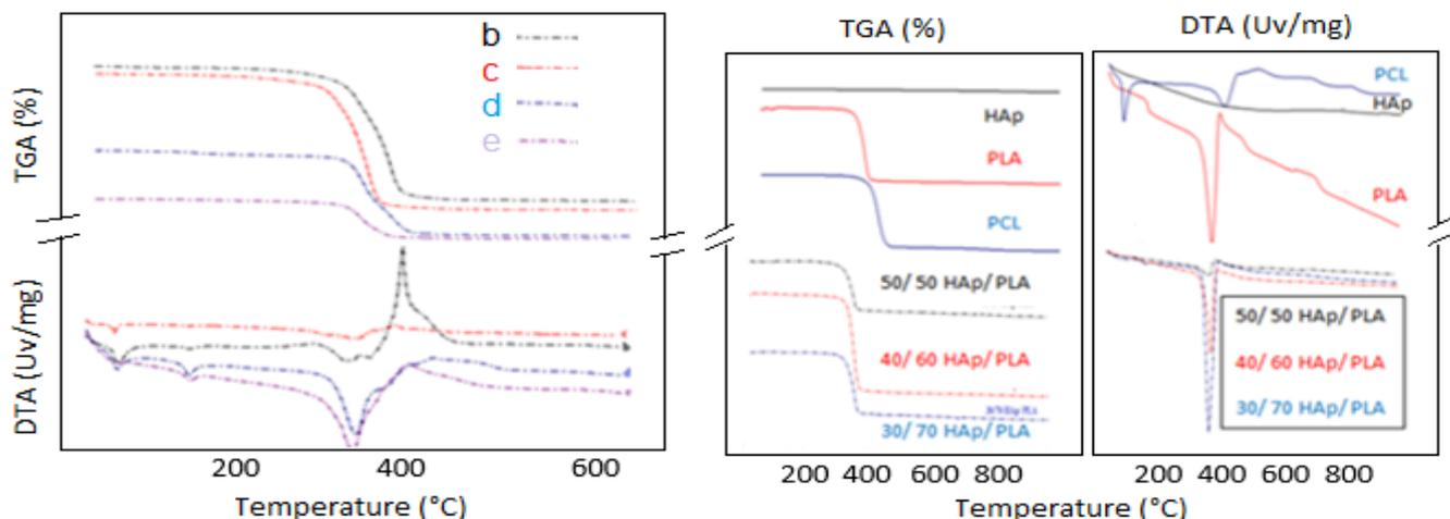
**Figure 6:** TGA (1) and DTA (2) curves of the composites HAp<sub>i</sub>/ PLA and HAp<sub>i</sub>/ PLA / PCL, with molar ratios of b = 50/30/20, c =50/10/40 d = 50/20/30 and e =50/40/10 (Heating rate: 10 °C / min).
