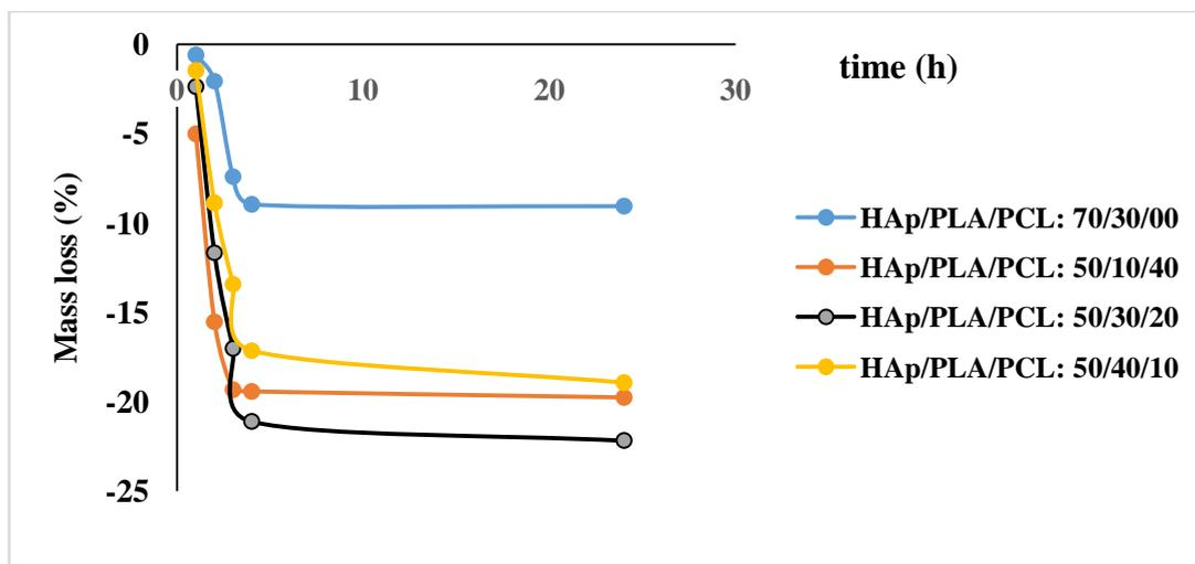
**Figure 7:** Biodegradability at 37 ° C of membranes HAp/PLA/PCL in PBS
