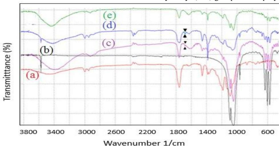
**Figure 2:** FTIR spectra of the HAp/PLA composite, with molar ratios: a=PLA, b= HAp, c = 70/30, d =60/40 and e=50/50.
