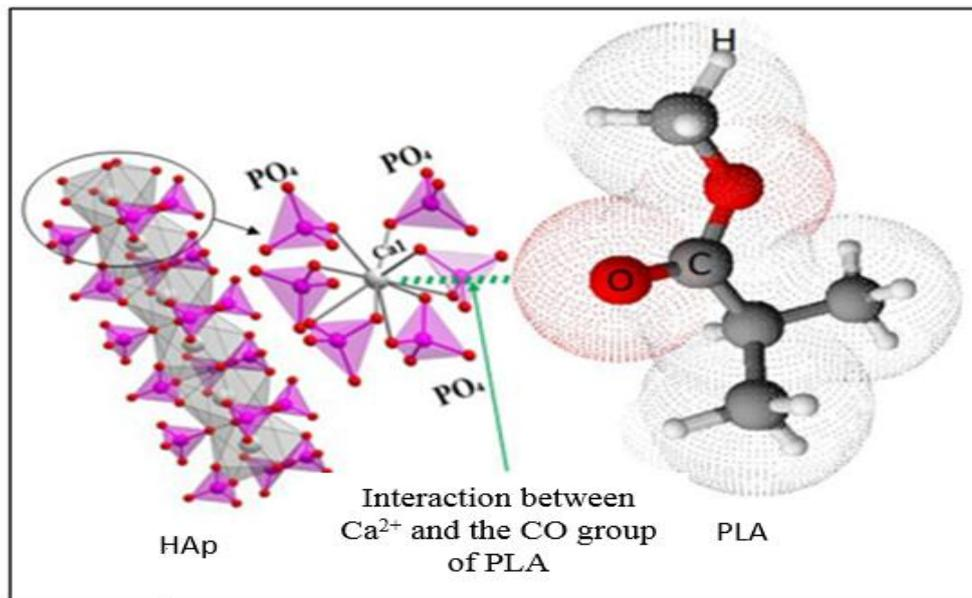
**Figure 3:** A schematic model of the complexation between the carboxyl groups of PLA and Ca<sup>2+</sup> of HAp.
