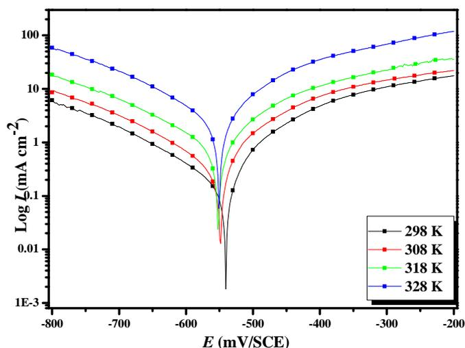
Figure 6. Potentiodynamic polarisation curves of carbon steel in 2M H<sub>3</sub>PO<sub>4</sub> in the presence of 5.10<sup>-4</sup> M of SMP at different temperatures
