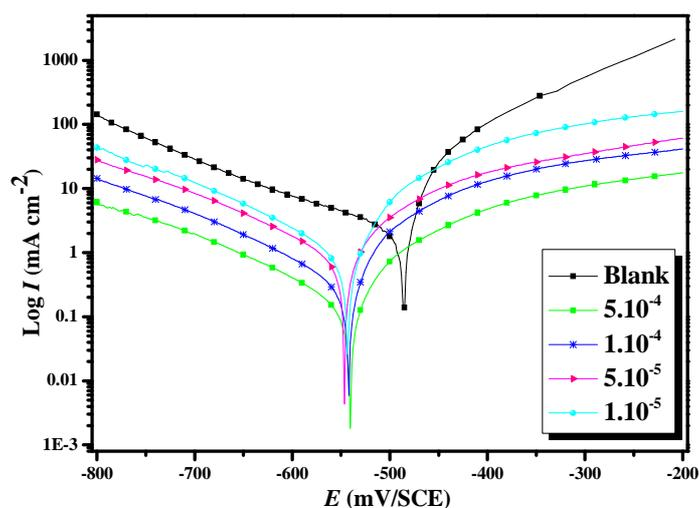
Figure 2. Potentiodynamic polarization curves of carbon steel in 2.0 M  $\text{H}_3\text{PO}_4$  in the presence of different concentrations of SMP
