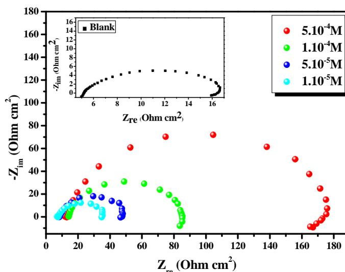
Figure 3. Nyquist diagrams of carbon steel with different concentrations of SMP at 298K
