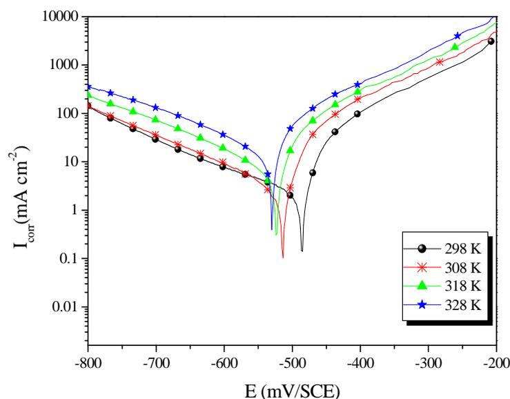
Figure 5. Potentiodynamic polarisation curves of carbon steel in 2M H<sub>3</sub>PO<sub>4</sub> at different temperatures
