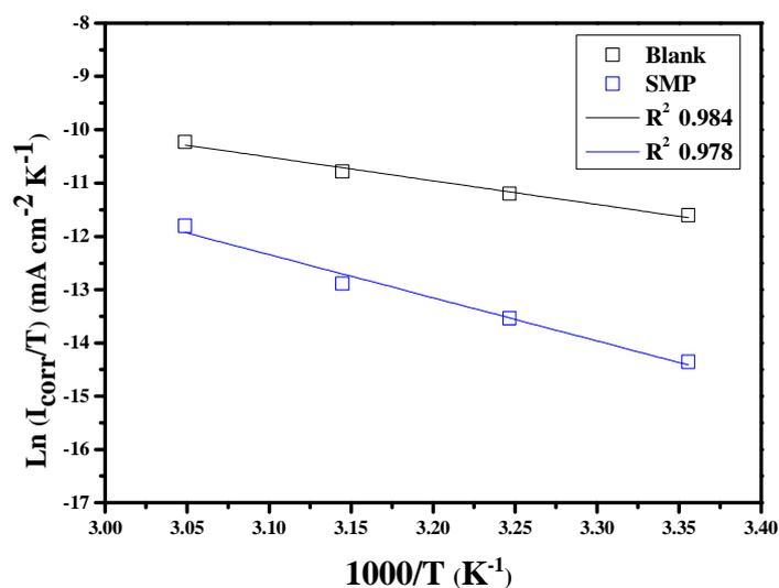
Figure 8. Arrhenius plots of carbon steel in 2.0 M H<sub>3</sub>PO<sub>4</sub> with and without 5.10<sup>-4</sup> M of SMP
