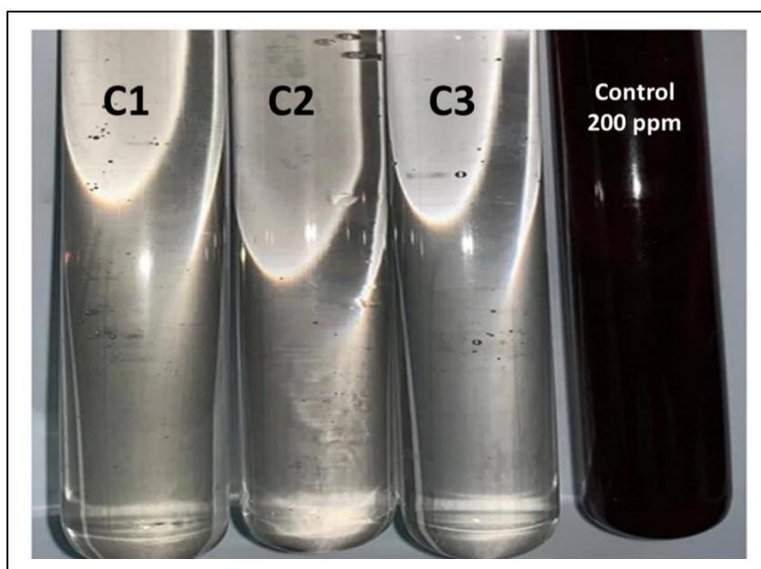
**Figure 3.** Pure effluents upon treating 200 ppm CV dye model molecule solution using  $Na_2S_2O_8$  oxidation agent in presence of  $Fe_3O_4$  nanoparticles.
