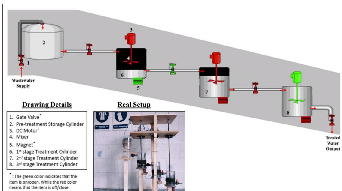
**Figure 2.** Schematic diagram of the magnetic wastewater treatment setup (drawn by using the Wondershare EdrawMax Software Version 10.5.2) and in-house built prototype.
