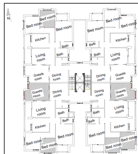
Figure 2. Al Maajeen sample for apartment building with selected rooms for measurements.
