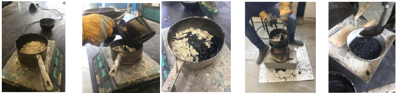
Figure 4. Mixing process of aggregates and bitumen with rubber
