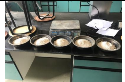
Figure 3. Preparation and distribution of aggregate samples
