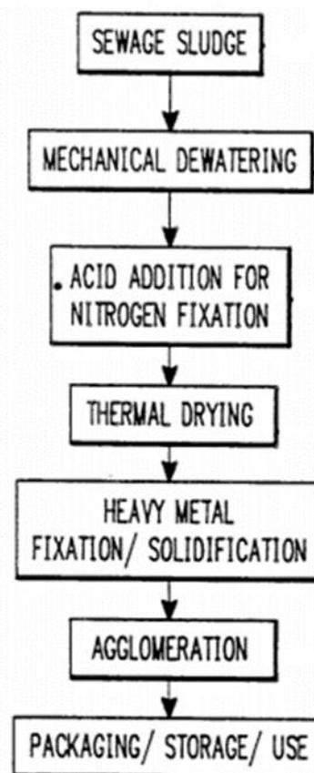
Figure 3: The fertilizer production process from Sewage sludge.
