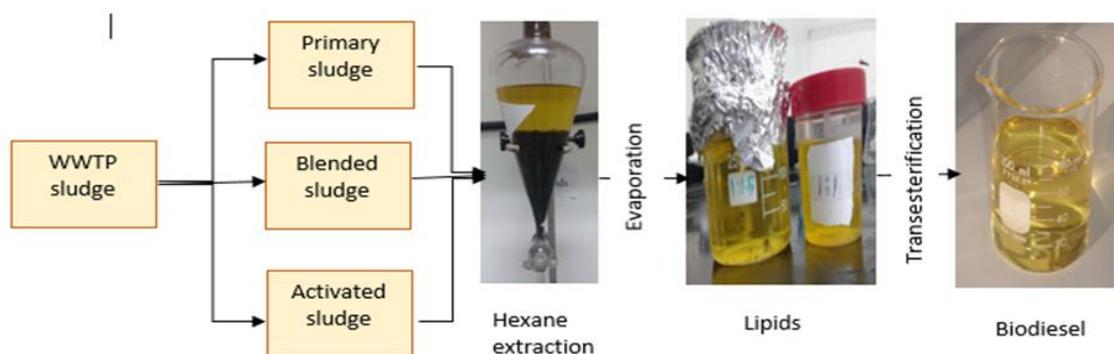
Figure 2: The whole process of Biodiesel production.
